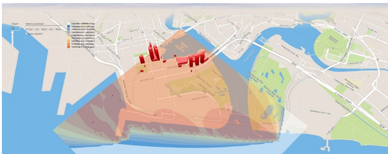
Fig. 5.7: Dispersion profile for atmospheric dispersion simulation of 30 ships with arbitrary cruising positions around waters surrounding Singapore at a height of 30 m.
