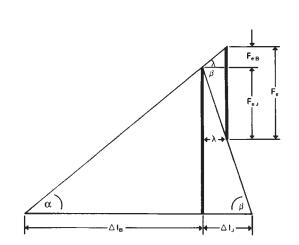
Fig. 7 Analysis of external load  $F_{\rm e}$  and derivation of Force Ratio  $\Phi.$
