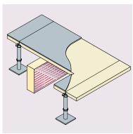
Fig.26 Access Floor FireStop Slab (typically directly under partition line)
