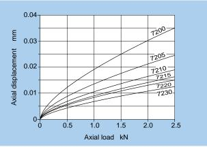
Fig. 17.2.7 Series 72 axial load and axial displacement
