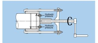
Fig. 15.20 Removal by hydraulic pressure
