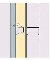
Fig.32 Sidewall cladding with Rockwool Cladding Roll and Rock-Lam Thermal Break strips - Weighted sound reduction index = Rw37 dB
