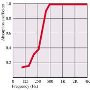
Rockwool Acoustic Acoustic Panel Wall Lining System on 50 mm battens - Average noise absorption coefficient: 0.90.
