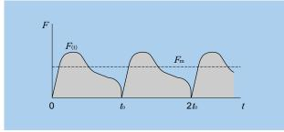
Fig. 4.9 Load that fluctuated as function of time
