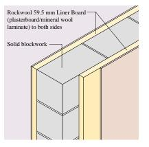
Fig.4 Rockwool Liner Board for upgrading existing cavity block party wall
