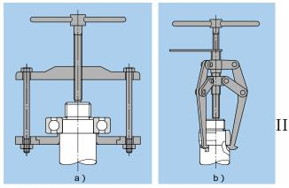
Fig. 15.15 Puller disassembly
