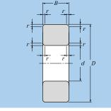
Fig. 5.1 Radial bearings (excluding tapered roller bearings)
