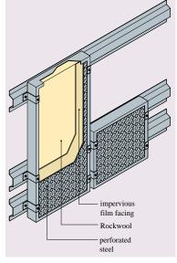
Fig.37 Rockwool Acoustic Element Casing: Single piece, aluminium, galvanised or stainless steel sheet formed into open-backed 'cassette'. Front face perforated with 3 mm dia holes, 33% open area.
