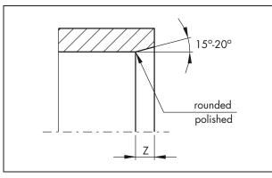
Figure 20 Lead-in chamfers for bores, tubes
