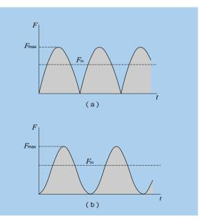
Fig. 4.11 Sinusoidal variable load
