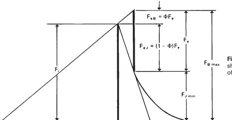
**Fig. 11 Modified joint diagram** shows nonlinear compression of joint at low preloads.
