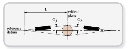
**Fig.11** Worst case angular misalignment =  $\alpha_1 + \alpha_2$
