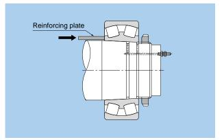
Fig. 15.23 Removal of bearing by hydraulic pressure
