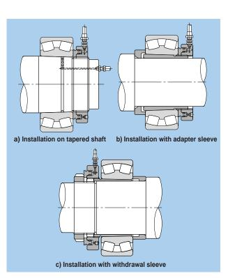
Fig. 15.9 Installation using hydraulic nut
