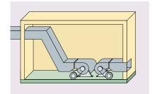
Fig.2 Acoustic lining to plant room where individual enclosure is impracticable. Lining formed using Rockwool Acoustic Elements (see
