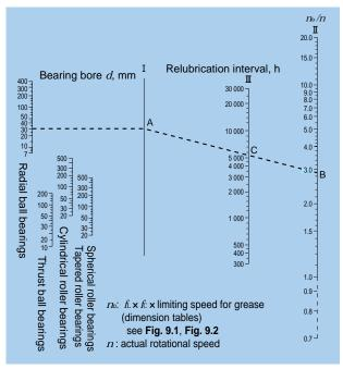
Fig. 11.2 Diagram for relubrication interval of greasing
