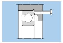
Fig. 15.19 Outer ring disassembly bolt
