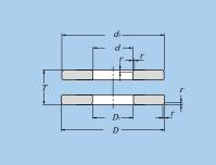
Fig. 5.3 Single direction thrust bearings
