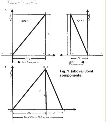
Fig. 2 Joint diagram is obtained by combining load vs. deformation diagrams of bolt and joints.
