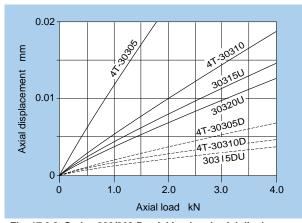
Flg. 17.3.3 Series 303/303 D axial load and axial displacement
