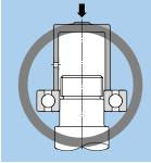
Fig. 15.3 Fitting sleeve pressure against inner ring
