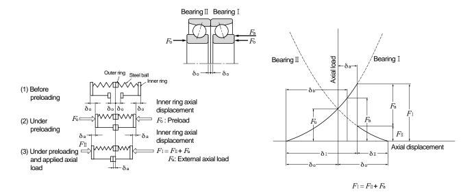
Fig. 8.2 Fixed position preload model diagram and preload diagram
