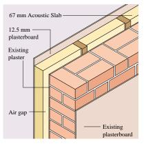
Fig.3 Upgrading an existing separating wall with access limited to one side only
