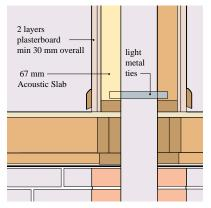
Fig.5 Rockwool Acoustic Slab or Timber Batts as insulation to timber framed separating walls.
