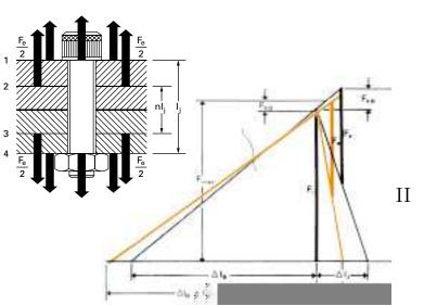
Fig. 8 Joint diagram shows effect of loading planes of  $F_e$  on bolt loads  $F_{eB}$  and  $F_{B max}$ . Black diagram shows  $F_{eB}$  and  $F_{B max}$  resulting from  $F_e$  applied in planes 1 and 4. Orange diagram shows reduced bolt loads when Fe is applied in planes 2 and 3.
