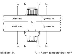
$T_2$  = Maximum operating temperature for
