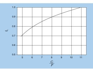
Fig. 9.1 Value of adjustment factor  $\hbar$  depends on bearing load
