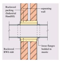
Fig.41 Reduction of structure borne noise at duct penetration - Rockwool Industrial Handfill / RW6 Slab
