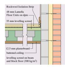
*Fig.21 Beam and block floor using Rockwool Lamella Floor Units*
