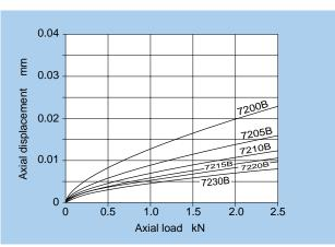
Fig. 17.2.8 Series 72 B axial load and axial displacement
