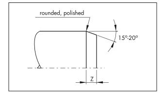
Figure 21 Lead-in chamfers for shafts, rods
