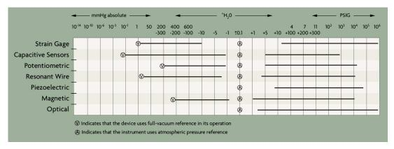
Figure 1: Electronic Pressure Sensor Ranges
