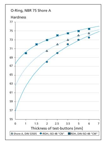
Figure 7 Ranges of hardness depending on sample thickness and test method
