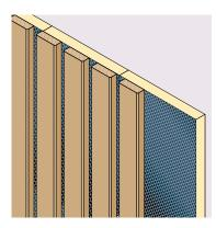
Fig.27 Rockwool Sound Absorption Board behind a slatted hardwood facing for acoustic control in an auditorium.
