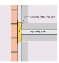
Fig.7 Acoustic Party Wall dpc for sound and fire resistance at separating walls
