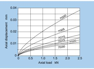
Fig. 17.2.4 Series 70 axial load and axial displacement
