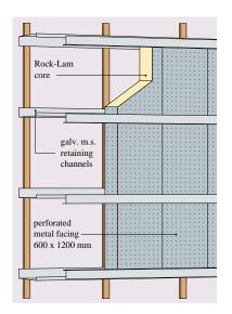
Fig.38 Rockwool Acoustic Panel Wall Lining System on 50 mm battens.
