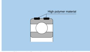
Diagram 1. Expansion compensating bearings
