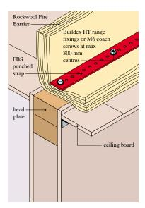
Fig.24 Fire Barrier above partition
