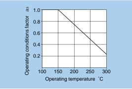
Fig. 3.2 Operating conditions factor according to operating temperature
