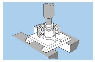
Fig. 15.16 Press disassembly
