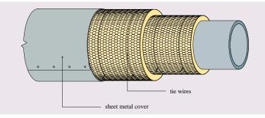
Fig.44 100 mm Wired Mat + 0.75 mm steel cladding without support rings. Pipe diameter 308 mm. The sound reduction achieved is shown in the graph below.
