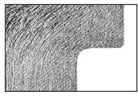
Controlled head forging, uniform grain flow, unbroken flow lines; makes heads stronger; minimizes failure in vital fillet area; adds to fatigue strength.
