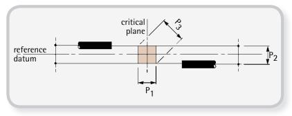
**Fig.13** *Maximum parallel error*  $=P_3$
