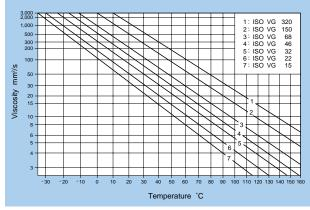
FIg. 11.5 Relation between lubricating oil viscosity and temperature
