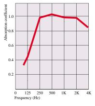
Rockwool Acoustic Element, standard size, fixed over a 50 mm cavity. Test method: ISO 354 (1985)
