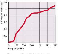
■ Rating according to EN ISO 11654: 1997 Weighted Sound Absorption Coefficient ∝<sub>w</sub> = 0.85 Test report BTC 10268A
