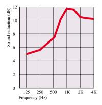
Typical noise reduction achieved through Rockwool absorbent lining to walls and ceilings enclosing noisy machinery
