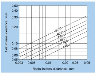
Fig. 17.1.2 Series 69 radial internal/axial internal clearances
