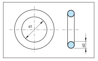
Figure 1 O-Ring dimensioning
