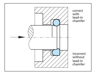
Figure 11 Rod installation with O-Ring
