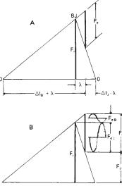
joint diagrams show external load Fe added (A), and external load divided into an additional bolt load F<sub>eB</sub> and reduction in joint compression F<sub>eJ</sub> (B). Joint diagram (C) shows how insufficient preload F<sub>i</sub> causes excessive additional bolt load F<sub>eB</sub>.
