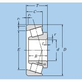
Fig. 5.2 Tapered roller bearings
