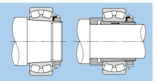
a) Installation on tapered bore b) Installation with adapter sleeve
