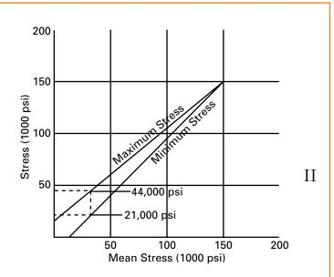
Fig. 18 – Goodman diagram of maximum and minimum operating limits for H-11 fastener at 800°F. Bolts stressed within these limits will give infinite fatigue life.
