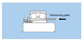
Fig. 15.21 Disassembly of bearing with adapter
