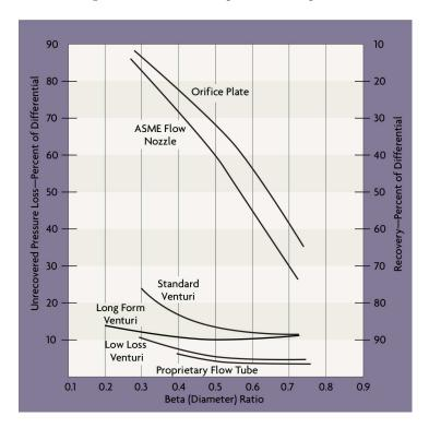
Figure 6: Pressure drop in Flowmeters
