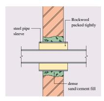
Fig.43 Alternative method with pipe sleeved through wall - using low density Rockwool packed tightly
