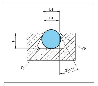
Figure 23 Installation in trapezoidal groove
