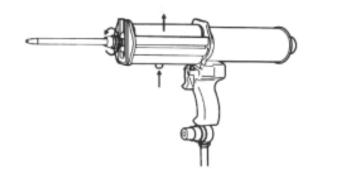
Fig.15 Handgun operated by compressed air
