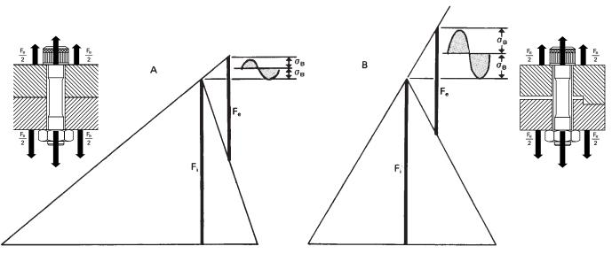
**Fig. 6** Joint diagram of a springy bolt in a stiff joint (A), is compared to a diagram of a stiff bolt in a springy joint (B). Preload  $F_i$  and external load  $F_e$  are the same but diagrams show that alternating bolt stresses are significantly lower with a spring bolt in a stiff joint.
