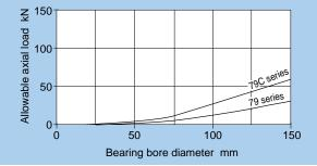
Fig. 17.4.3 Allowable axial load for angular contact ball bearings (79, 79C series)
