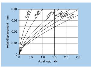
Fig. 17.2.3 Series 70 C axial load and axial displacement
