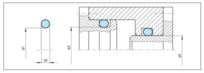
Figure 18 Radial installation, static and dynamic
