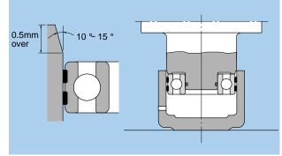
Diagram 2. Fitting method and housing inner diameter chamfer
