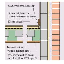
Fig.20 Beam and block floor using Rockwool Rockfloor on levelling screed
