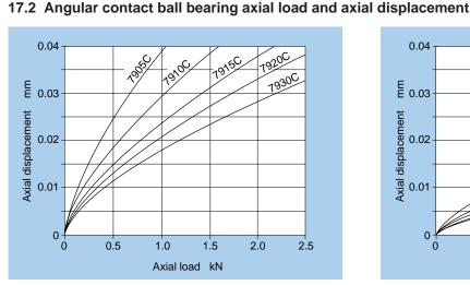
Fig. 17.2.1 Series 79 C axial load and axial displacement
