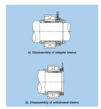
fig. 15.24 Disassembly using hydraulic nut
