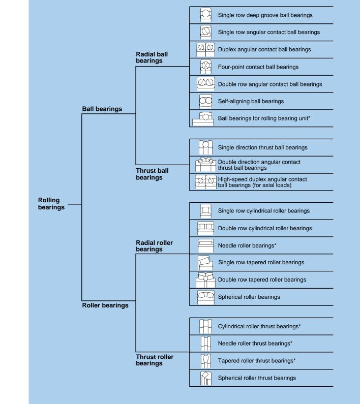
Fig. 1.2 Classification of rolling bearings
