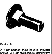
A warm-headed truss square shoulder bolt of Type 384 stainless. By using warm heading, less forming pressure was required on the die resulting in increased tool life.
