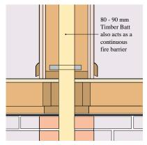
Fig.6 Alternative method of acoustic insulation in timber framed separating wall using Rockwool Timber Batts in the cavity
