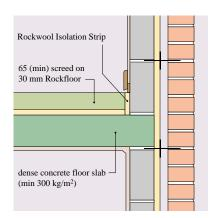
Fig.23 Dense concrete floor using Rockwool Rockfloor under screed
