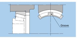
Fig. 15.18 Extraction groove for outer ring disassembly
