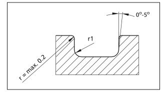
Figure 24 Groove specifications
