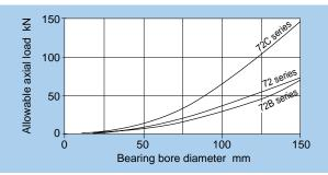
Fig. 17.4.2 Allowable axial load for angular contact ball bearings (72, 72B, 72C series)
