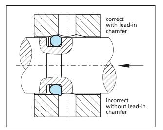
Figure 13 O-Ring installation over transverse bores
