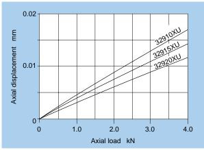
Fig. 17.3.2 Series 329 axial load and axial displacement
