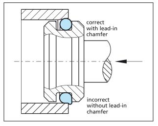
Figure 12 Piston installation with O-Ring
