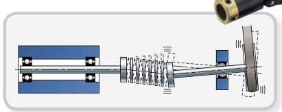
**Fig.20** A semi-floating shaft located by a self-aligning bearing at one end and a multi-stage bellows at the other. The coupling reacts to fluctuating tension in the belt by allowing lateral oscillations in the shaft.
