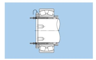
Fig. 15.25 Disassembly using hydraulic withdrawal sleeve
