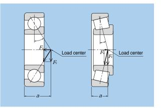
Fig. 4.12 Pressure cone apex and axial component force
