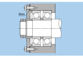
Fig. 15.14 Internal clearance adjustment using shims
