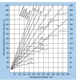
Fig. 15.5 Temperature required for heat-fitting inner ring
