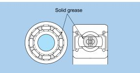
Fig. 11.3 Deep groove ball bearing with spot-pack solid grease (Z shield) (Standard for deep groove ball bearings)
