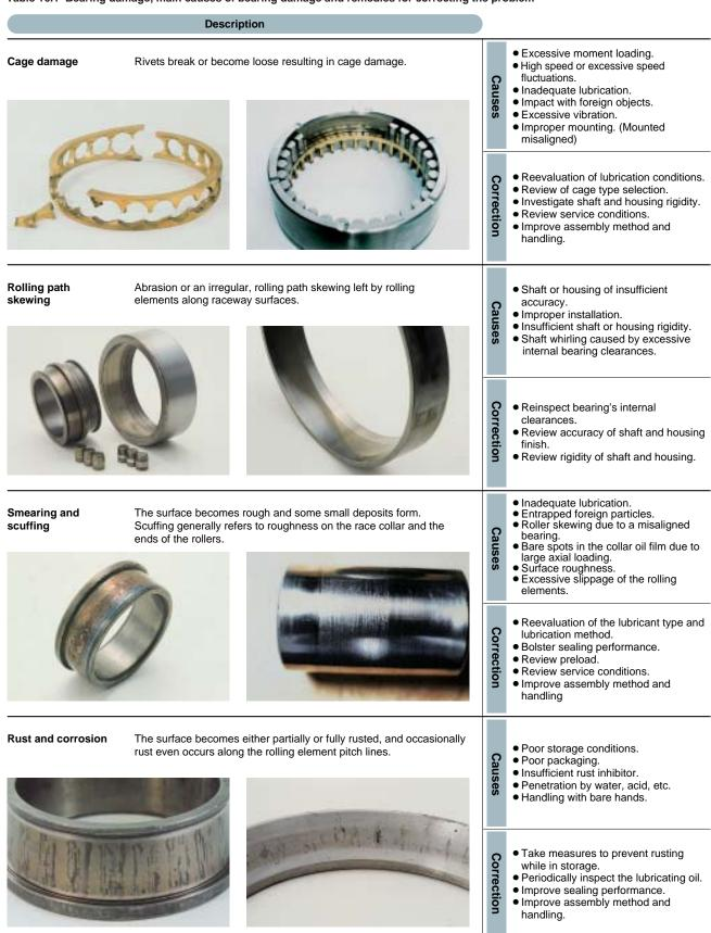
Table 16.1 Bearing damage, main causes of bearing damage and remedies for correcting the problem
