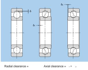
Fig. 8.1 Internal clearance
