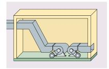
Fig.36 Acoustic lining to plant room where individual enclosure is impracticable. Lining formed using Rockwool Acoustic Elements (see
