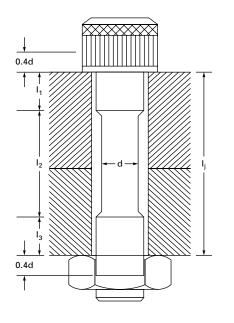
Fig. 4 Analysis of bolt lengths contributing to the bolt spring rate.
