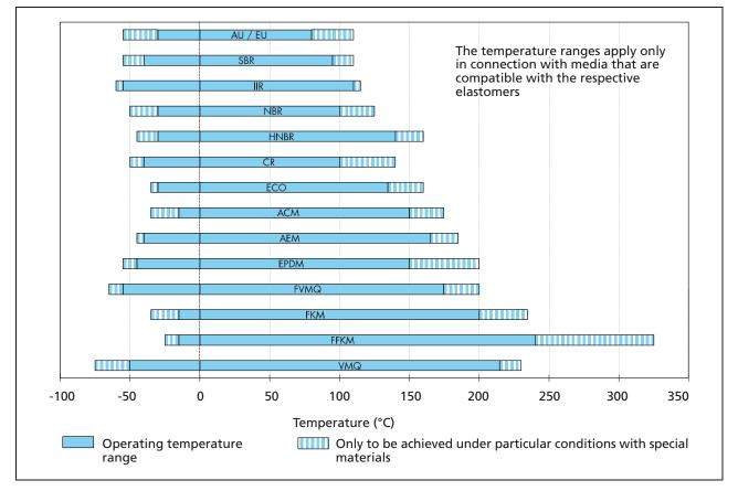
Figure 4 Temperature range of various elastomers
