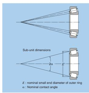
Fig. 1.3 Tapered roller bearings
