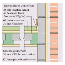
Fig.23a Screeded beam and block floor
