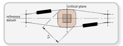
**Fig.14** Worst case radial error  $r_2 = p_3 + r$
