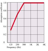
Typical absorption coefficients -Rockwool 67 mm Acoustic Slab
