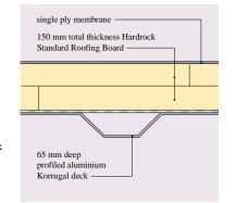
Fig.31 Flat roof detail, Stansted Airport, with Rockwool Hardrock Roofing Board - Sound reduction index = 44 dB.
