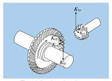
Fig. 4.4 Loads on bevel gears
