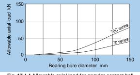
Fig. 17.4.4 Allowable axial load for angular contact ball bearings (70, 70C series)
