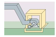
Fig.35 Isolation of plant noise source by acoustic treatment of base and individual enclosure. Enclosure formed by steel faced partition with perforated inner sheet and incorporating Rockwool Rigid Slab (typically RW3).
