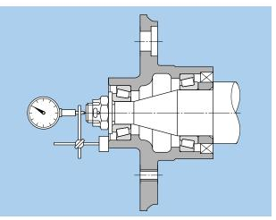
Fig. 15.13 Measurement of axial internal clearance adjustment
