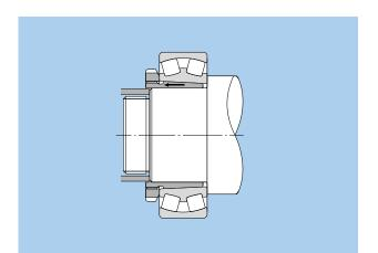
Fig. 15.22 Disassembly of bearing with withdrawal sleeve
