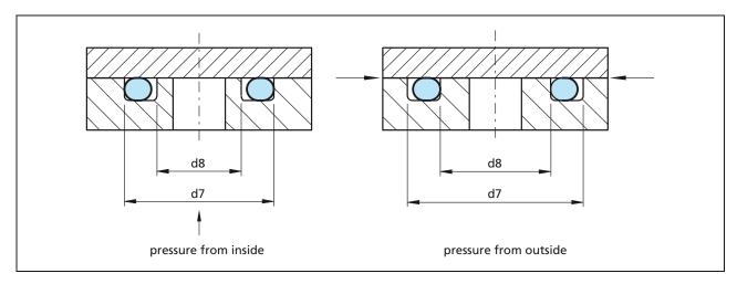
Figure 19 Axial installation, static
