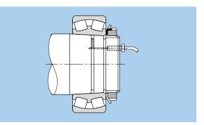
Fig. 15.8 Installation utilizing oil injection
