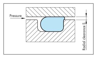
Figure 22 Radial clearance "S"
