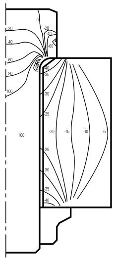
**Fig. 5** Lines of equal axial stresses in a bolted joint obtained by the axisymmetric finite element method are shown for a 9/16–18 bolt preloaded to 100 KSI. Positive numbers are tensile stresses in KSI; negative numbers are compressive stresses in KSI.
