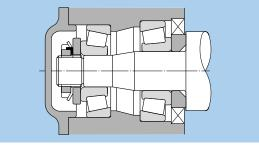
Fig. 15.12 Axial internal clearance adjustment
