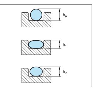
Figure 9 Illustration of the compression set
