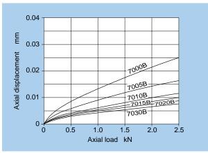
Fig. 17.2.5 Series 70 B axial load and axial displacement
