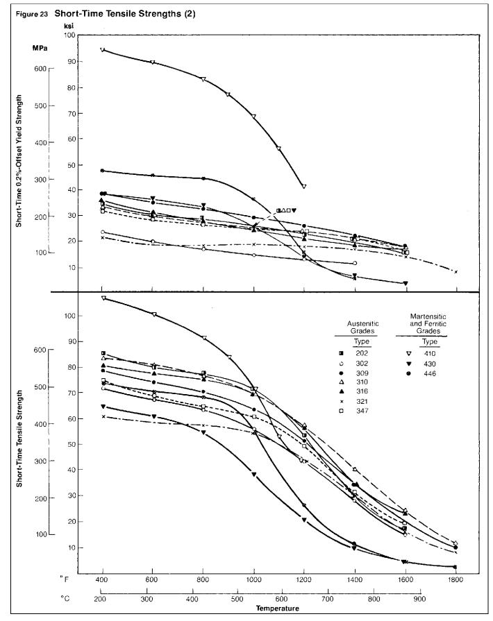
Typical short-time tensile strengths of various standard stainless steels at elevated temperature. All steels were tested in the annealed condition except for the martensitic Type 410, which was heat treated by oil quenching from 1800 °F (982 °C) and tempering at 1200 °F (649 °C).
