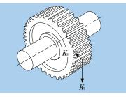
Fig. 4.1 Spur gear loads
