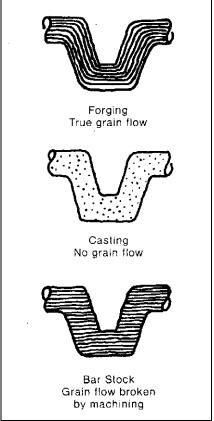
A unique feature of forgings is that the continuous grain flow follows the contour of the part, as illustrated by the top drawing in Exhibit 5. In comparison is the random grain structure of a cast part (center) and the straight-line orientation of grain in a machined part (bottom). From this difference stem secondary advantages inherent in forged stainless steels as follows:
