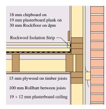
Fig.19 Timber joisted floor using Rockwool Rockfloor and Rockwool Rollbatt
