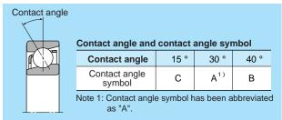
Table 1.4 Configuration of double row angular contact ball bearings
