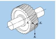
Fig. 4.2 Helical gear loads
