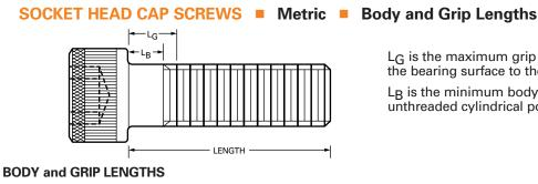
$\mathsf{L}_G$  is the maximum grip length and is the distance from the bearing surface to the first complete thread.
