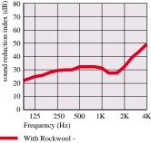
Weighted sound reduction index: R<sub>w</sub> 32 dB Test report No. AC97-216 Test No.1
