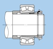
c) Installation using withdrawal sleeve
