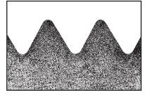
Contour-following flow lines provide extra shear strength in threads, resist stripping and provide high fatigue resistance. The large root radius UNBRAKO socket screw development doubles fatigue life compared to flat root thread forms.
