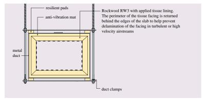
Fig.39 Internal acoustic lining to attenuate duct-borne noise - Rockwool RW3 and tissue lining on the exposed side
