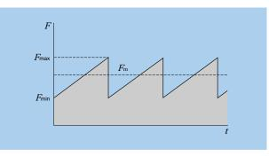
Fig. 4.10 Linear fluctuating load
