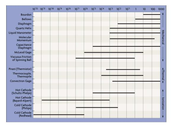
Figure 2: Vacuum Gauge Measurement Ranges
