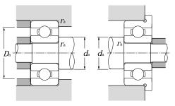
With flanged outer ring and double shield (FL...ZZ)
