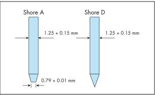
Figure 5 Indentor according to Shore A / D
