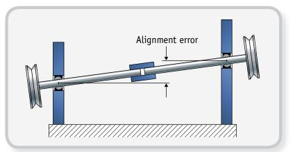
**Fig.21** Shafts located by self-aligning bearings can float into perfect alignment for connection with a solid coupling.
