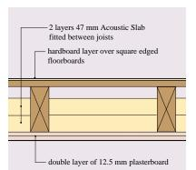
Fig.18 Upgrading the airborne sound insulation of a fixed timber floor using 2 layers of 47 mm Rockwool Acoustic Slab.
