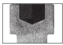
Accurate control of socket depth gives more wrench engagement than other screws, permits full tightening without cracking or reaming the socket, yet provides ample metal in the crucial fillet area for maximum head strength.
