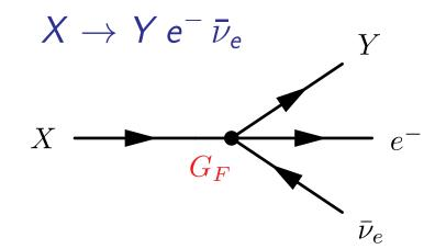
No "propagator" – absorb the effect of the exchanged W boson into an effective coupling strength given by the Fermi constant  $G_F = 1.166 \times 10^{-5} \text{ GeV}^{-2}$ .
