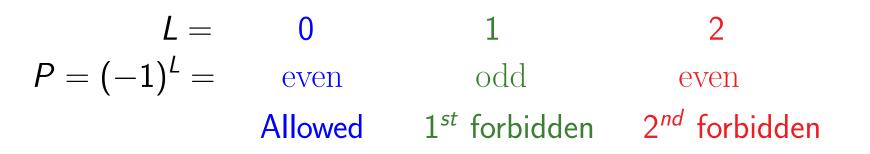
Transition probabilities for L > 0 are small  $\Rightarrow$  forbidden transitions (really means "suppressed").
