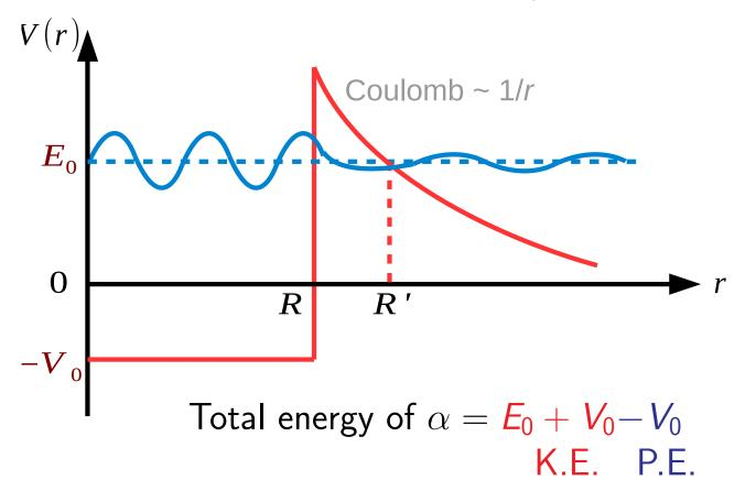
Classically,  $\alpha$  particle cannot enter or escape from nucleus. Quantum mechanically,  $\alpha$  particle can penetrate the Coulomb barrier
