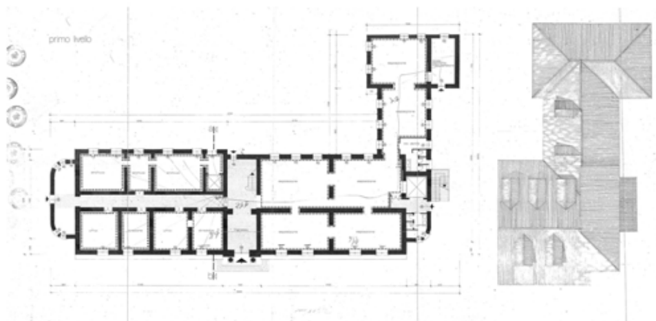
Figure 5: The main building, ground floor plan and roof plan details (survey by Studio Eng. G. Scarnati)
