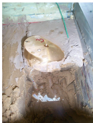
Figure 11 (c): Pile 3 after the earthquake.
