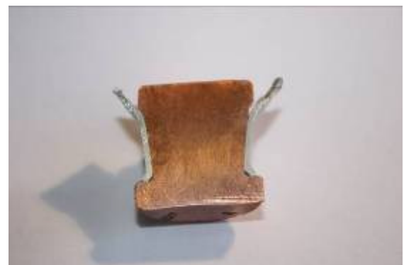
Fig 20: EMPT welded aluminium-copper transition joint ( \phi 25\text{mm} dia.)
