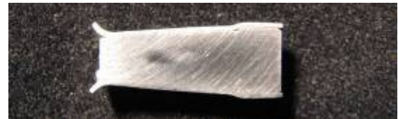
Fig 19: EMPT welding of the ferritic-martensitic steel T91 for nuclear fuel rods ( \phi 8\text{mm} )
