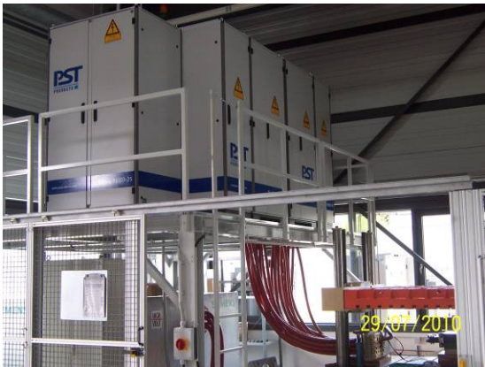
Fig 22 Heavy-duty EMPT BlueWave system PS103-25 with 103kJ energy at 25kV voltage
