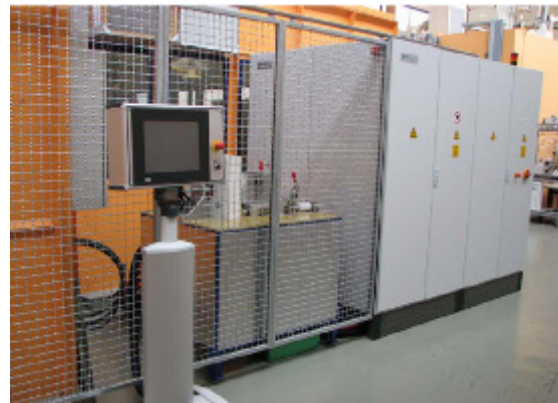
Fig 25: Heavy-duty EMPT BlueWave system PS100-10 with 100kJ energy at 10kV voltage
