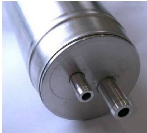
Fig 3: EMPT welding of a pressure vessel for air condition systems (ø75mm dia. aluminium)
