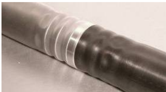
Fig 2: EMPT crimping of aluminium and steel tubes onto an aluminium node for an IP beam
