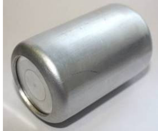
Fig 9: EMPT hemming of a pressure vessel for aluminium shock absorbers
