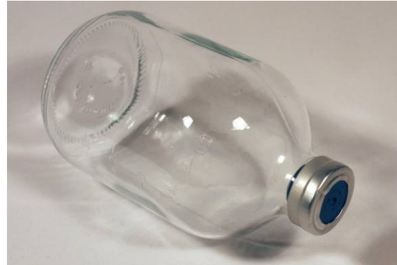
Fig 13: Aluminium lid EMPT crimped onto pharmaceutical glass vial
