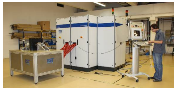
Fig 24: Heavy-duty PS96-16 BlueWave System by PSTproducts with 96kJ at 16kV for use in the industrial environment of the world's largest aluminium extrusion company Sapa
