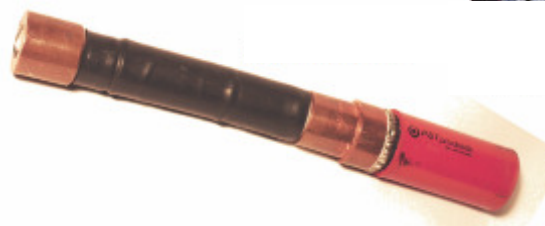
Fig 14: EMPT crimped high current cable: copper-copper and copper-steel-copper joints
