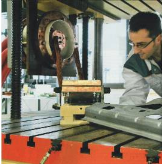
Fig 21: EMPT cutting of automotive sheets at Fraunhofer IWU in Chemnitz using a PSTproducts BlueWave coil
