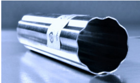
Fig 11: EMPT formed spline ( \phi 40\text{mm} )
