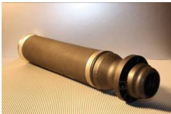
Fig 12: EMPT crimped air suspension
