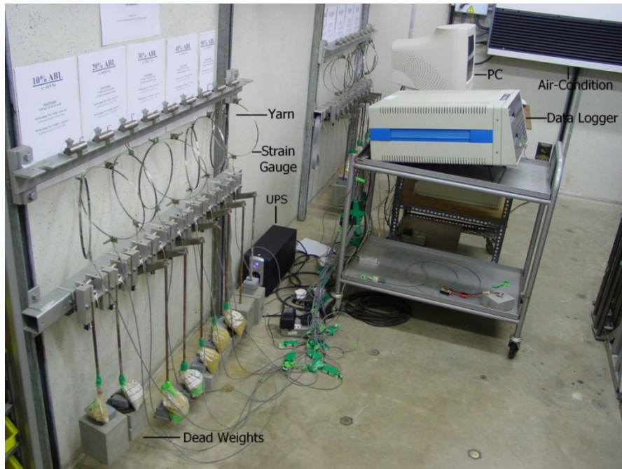
Figure 3 Experimental set up of the creep experiment
