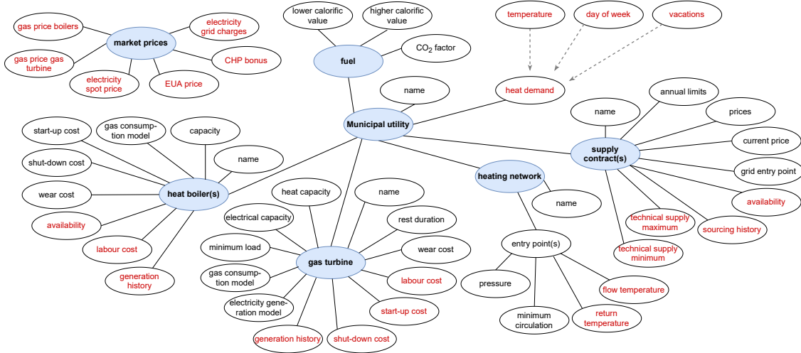
Figure 2: Class structure of virtual municipal utility representation: blue shaded elements represent classes, black elements denote constant attributes, and red elements represent time series attributes. Dashed arrows indicate the influence of external variables on total heat demand.
