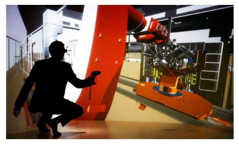
Virtual prototype within the immersive CAVE (Cave Automatic Virtual Environment) at The Manufacturing Technology Centre (MTC) in Coventry
