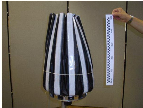
Figure 5.3: First step of zig-zag folding.
